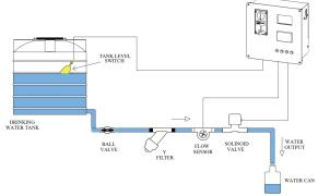
Note: The solenoid valve and flow sensor should be installed in the correct direction, as close as possible to the water output  $\frac{1}{2}$
